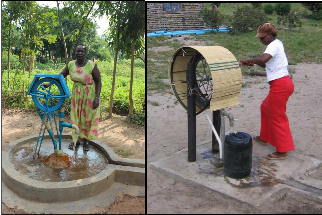
Figure 4-4. (a) Family Rope Pump in use in Gulu, Uganda (photo: J.D. Carpenter); (b) Family Rope Pump in use in South Africa (MacCarthy, 2004)
